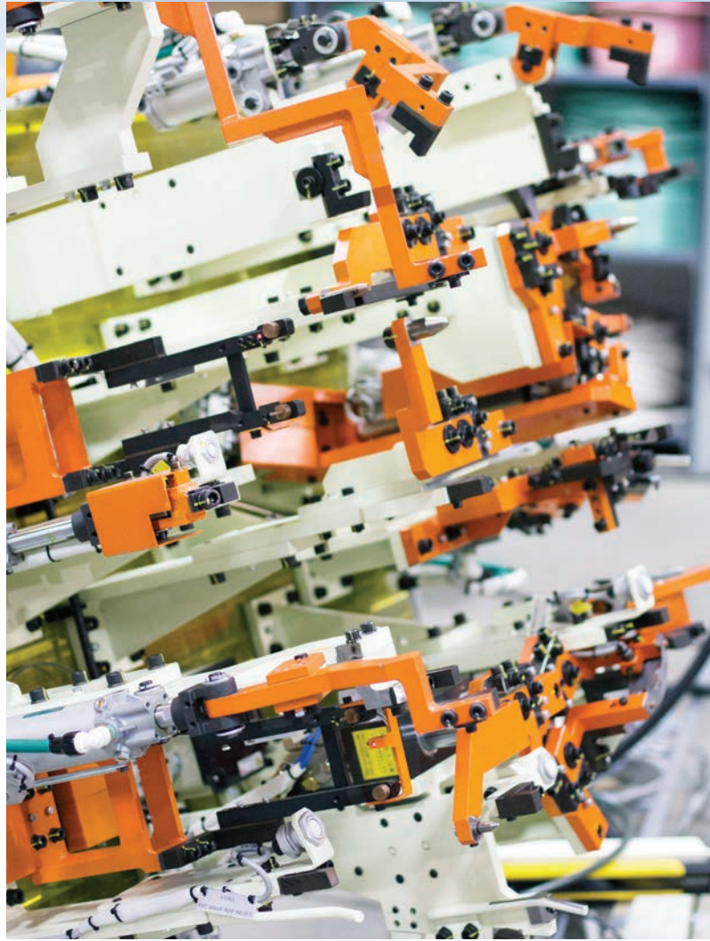
Door Inner Jig ▶
