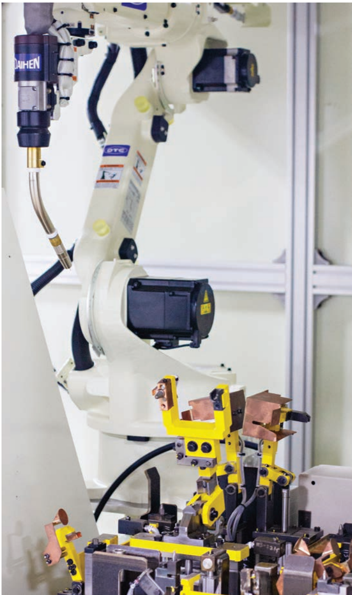
◀ Arc Weld Booth
